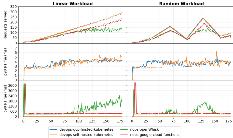
Fig. 5: /movies API endpoint performance comparison results for different deployment strategies along with two different methods by which these two can be achieved on two different workload patterns for two metrics: number of requests served and P90 response time.
