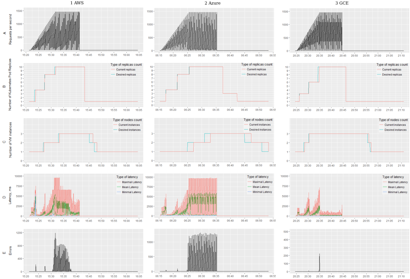
Figure 1. The results of the multilayered autoscaling evaluation for the linear increase and constant pattern. Rows: A) Number of requests sent; B) Desired and current amount of Kubernetes pods; C) Desired and current amount of VM instances; D) Minimal, Mean, and Maximal latency; E) Number of errors.
