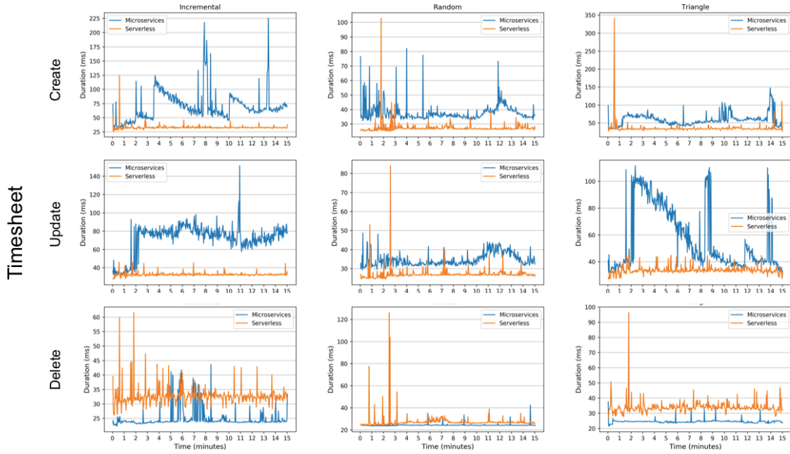
Figure 6: Comparison of percentile95 response time in Timesheet module for both microservices and serverless deployment at different workload patterns.
