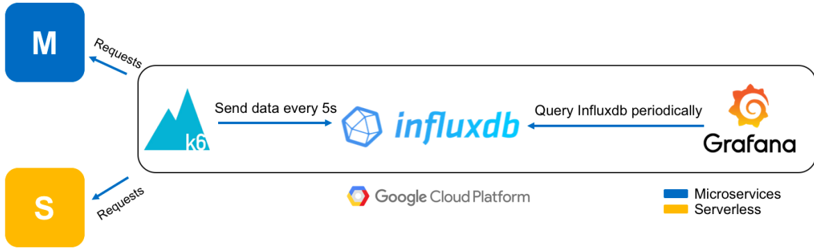
Figure 4: Overall evaluation system design for evaluating each of the strategies using the k6 as the load generator, influxdb for storing the data and grafana for real time visualization deployed on the Google Cloud Platform.
